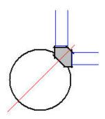
Cut the top of the poles so that shear the loads are embedded. Bolt through the post at 3" end distance and 9" centers to make the braket integral with the posts themselves.
